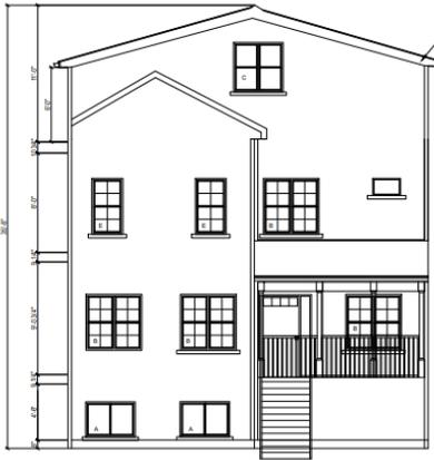
Building deviated from initially depicted roof construction, and constructed top floor with 6' walls no dormer conditions.
